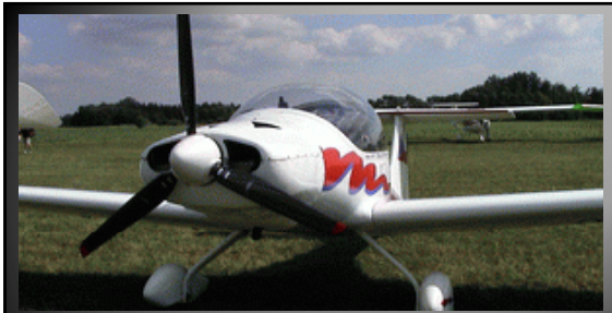
Action: the propeller pushes the air back >> REACTION: The plane goes forward
