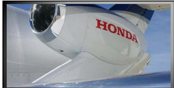
Action: Jet engine pushes exhaust gasses back >> REACTION: The plane goes forward
